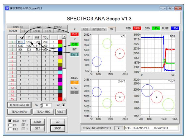
Now press the **SEND** button again to inform the sensor about the taught color. Then activate the **GO** mode again. When the sensor recognises a row vector (color), the corresponding row number is visualised on the software interface under **C-No**:. A value of 255 means that none of the taught colors were recognised.
